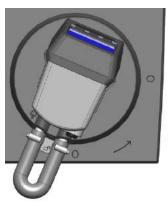
3. Rotate the Temperature Controller counterclockwise until the Locking Tab engages the indent on the top deck.
