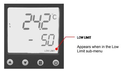
To Access: Press the lakey until LOW LIMIT appears on the display.
