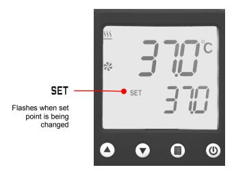
**To Change:** Press the or key. The word "SET" will begin flashing. Continue holding or repeatedly press or until the desired set point temperature is displayed.
