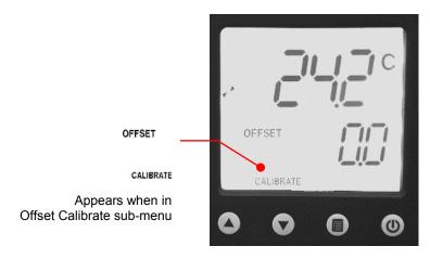
To Access: Press the likey until OFFSET CALIBRATE appears on the display.
